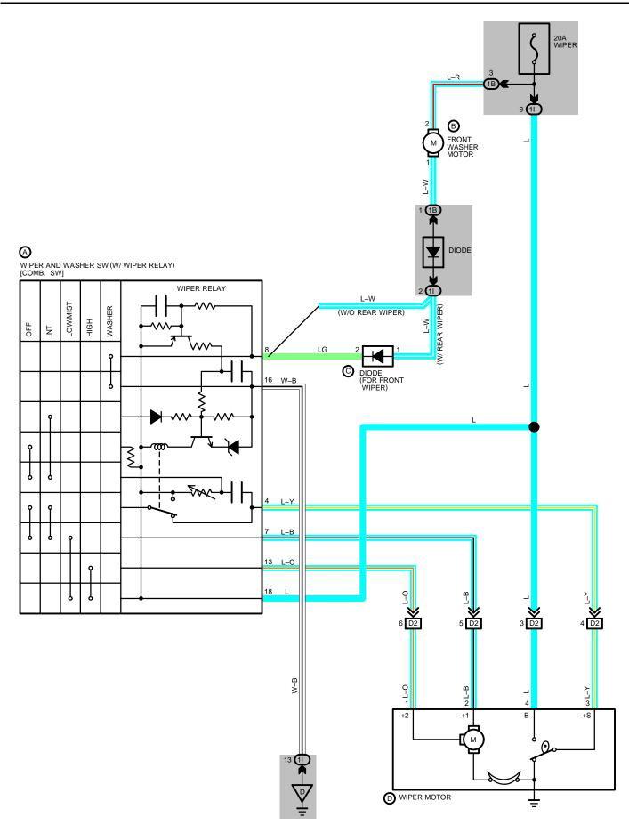
WITH THE IGNITION SW TURNED ON, THE CURRENT FLOWS TO TERMINAL 18 OF THE WIPER AND WASHER SW, TERMINAL 2 OF THE WASHER MOTOR AND TERMINAL 4 OF THE WIPER MOTOR THROUGH THE WIPER FUSE.
